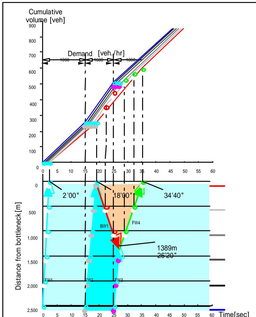
Fig. 41 Traffic condition transition diagram upstream of bottleneck (below) and through volume cumulative curve at each observation section (above)
