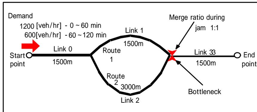
Fig.48 Example of verification data set for reproducibility of route selection behavior
