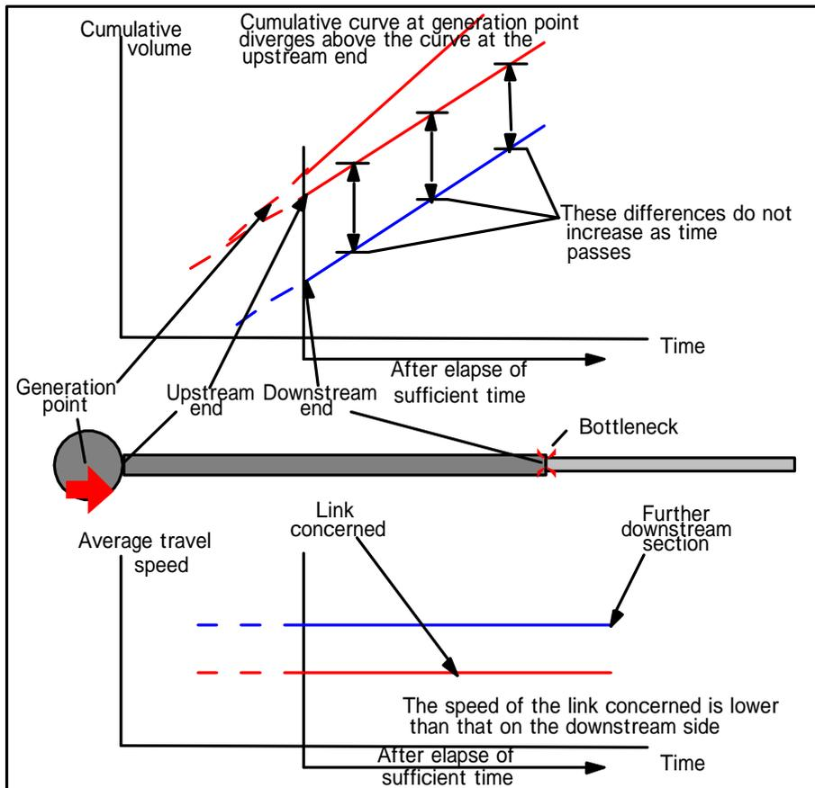
Fig.A1-2 Conceptual view when the flow in a traffic jam is in a steady state
