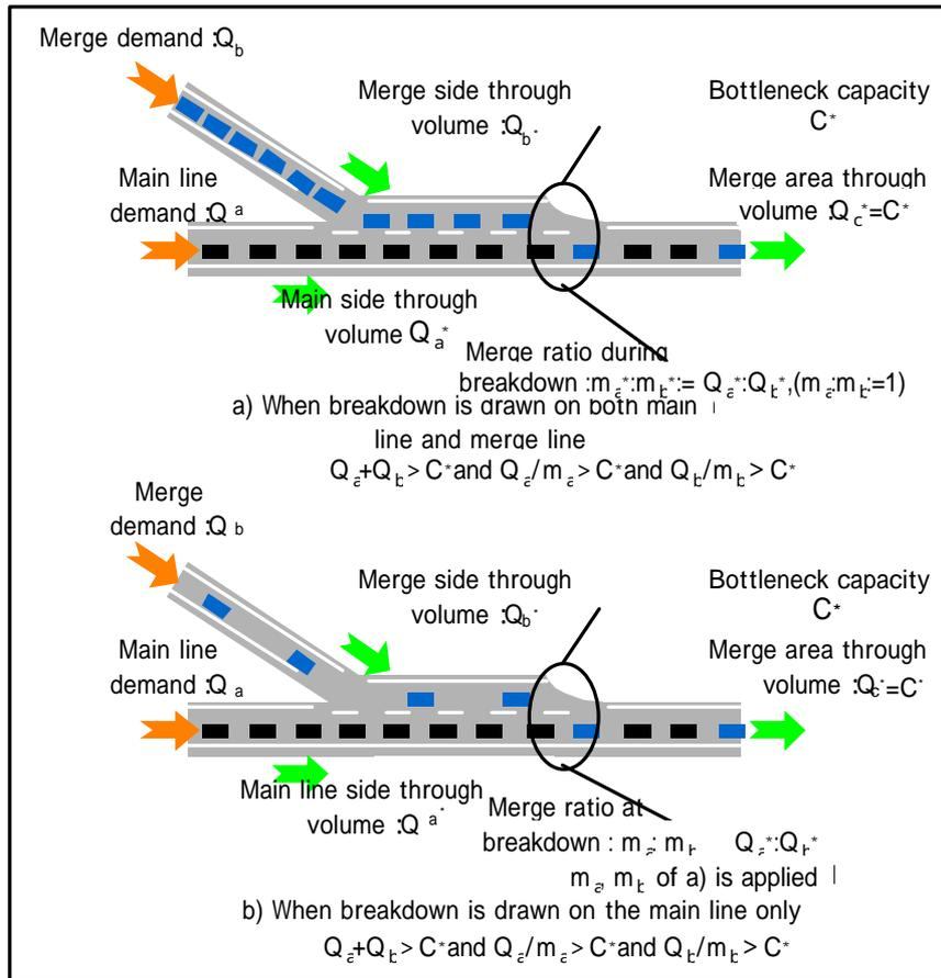
Fig.6 Difference of breakdown drawing at merge area depending on the capacity and merge/diverge ratio
