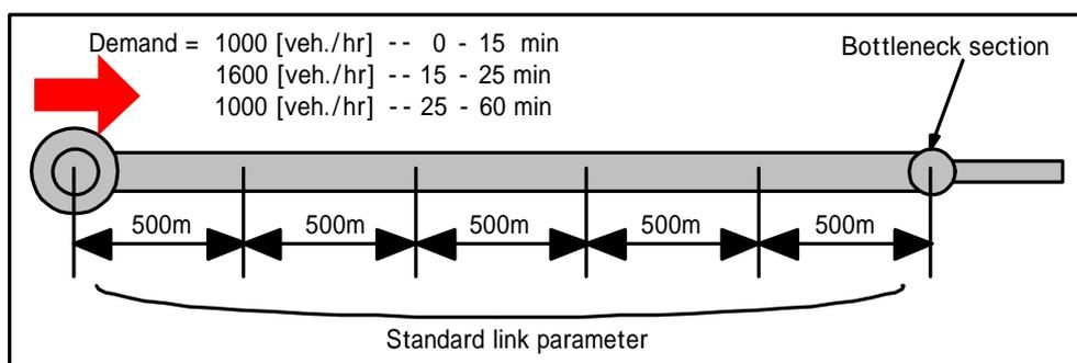
Fig.39 Verification data set for spreading vehicles and eliminating jams
