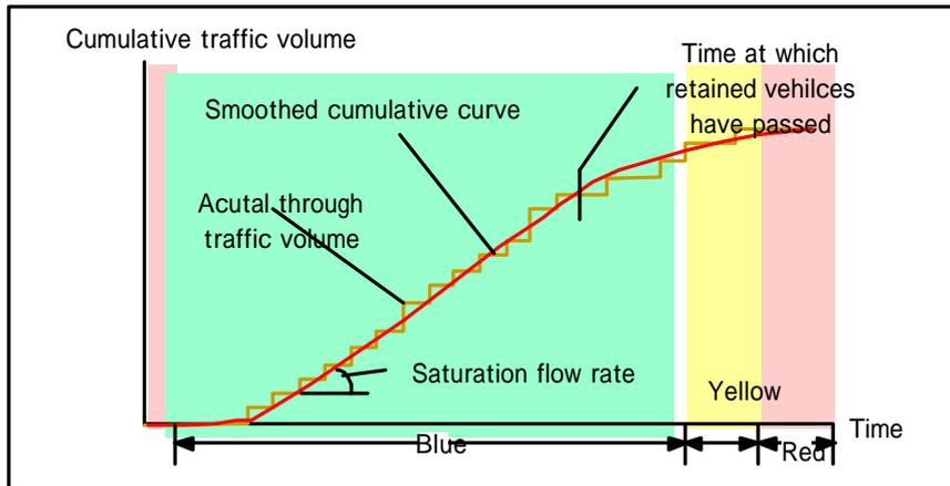
Fig.3 Conceptual view of one-cycle outflow pattern at a signalized intersection
