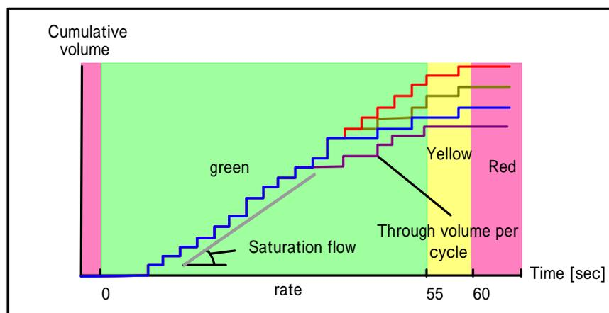
Fig.38 Saturation flow rate observed at the link downstream end
