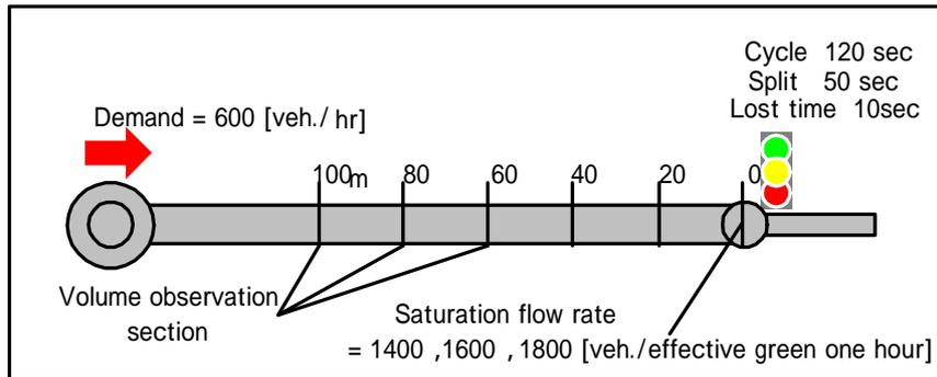
Fig.22 Verification data set for reproducibility of start/stop wave according to signal
