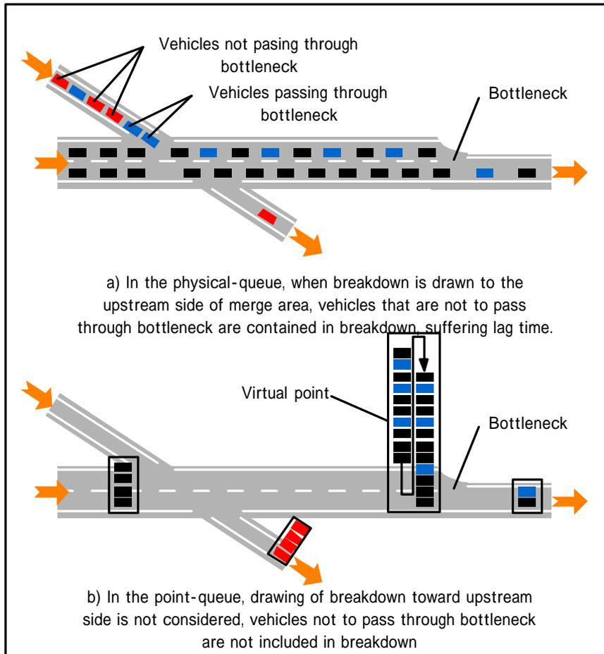
Fig.4 Difference between point-queue and physical-queue
