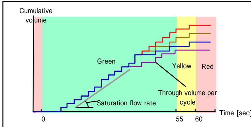
Fig.18 Saturation flow rate observed at link downstream end
