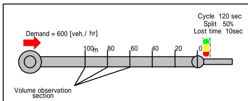
Fig.42 Verification data set for start/stop wave under control of signal
