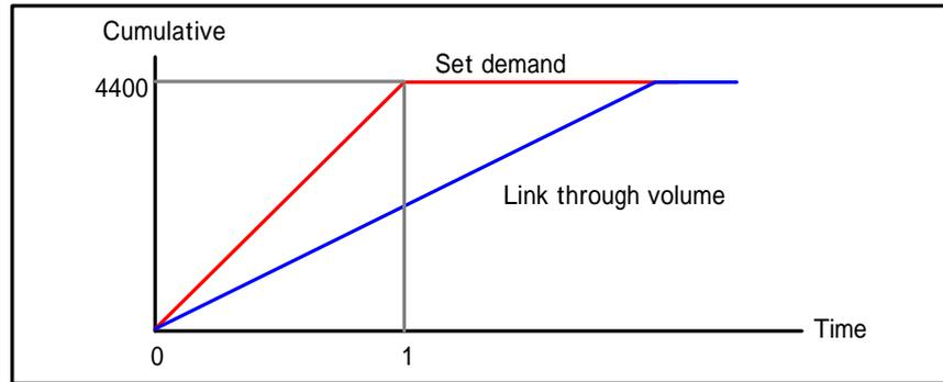
Fig.34 Volume cumulative curve projected when the 4400veh/hr demand is given
