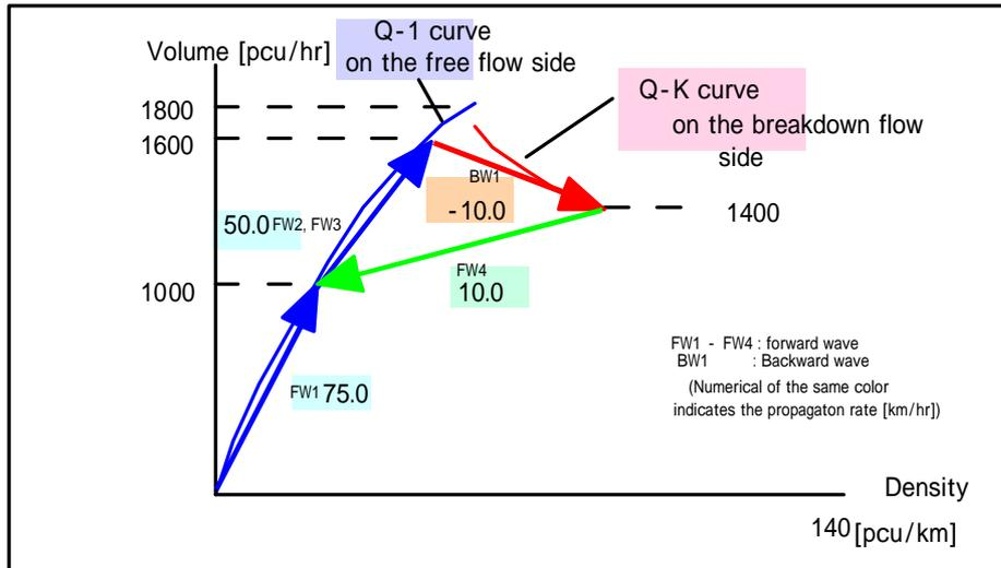
Fig.40 Shock wave propagation rate determined from Q-K curve
