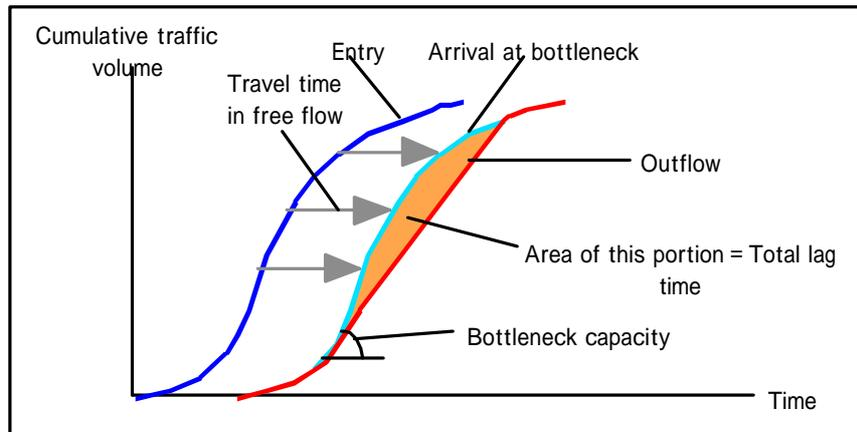
Fig.2 Conceptual view of lag time evaluation using Point-queue
