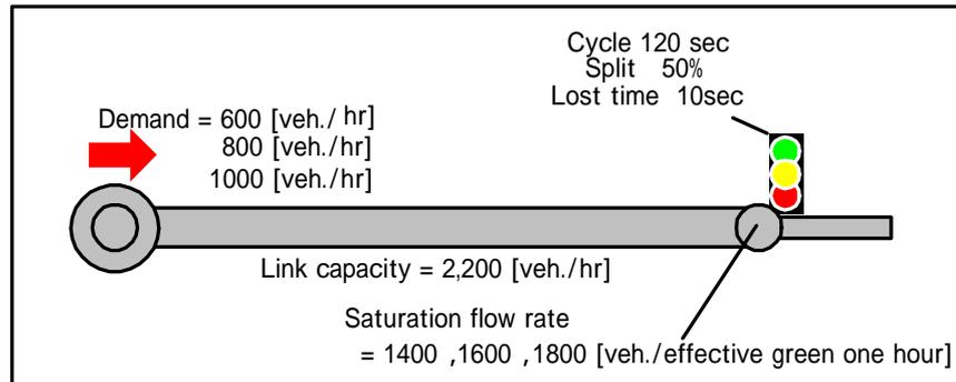
Fig.17 Verification data set on reproducibility of saturation flow rate at link downstream end
