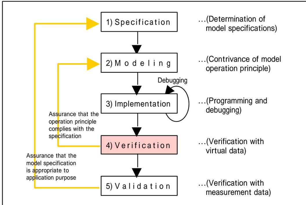
Fig.1 General simulation-model development process
