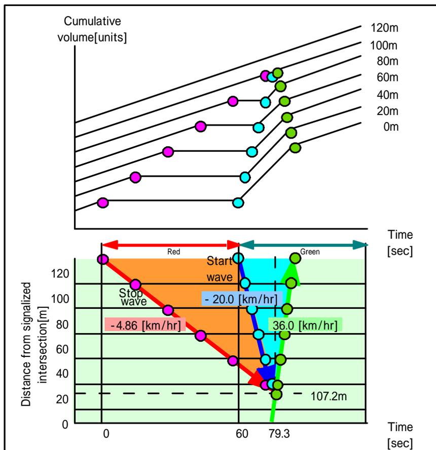
Fig.24 Start and stop wave propagation manner and cumulative volume at each point
