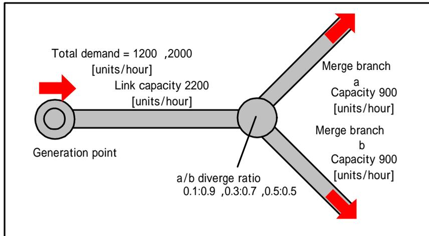
Fig.26 Verification data set for reproducibility of diverge area capacity
