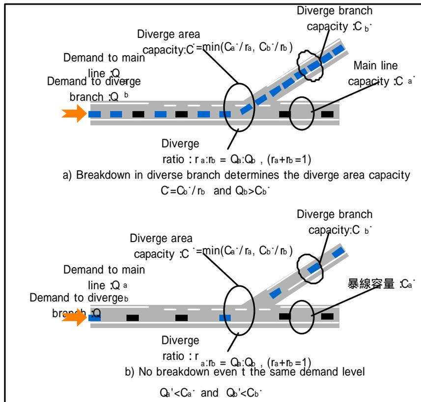
Fig.7 Difference in breakdown depending on difference in capacity and diverge ratio in the diverge area
