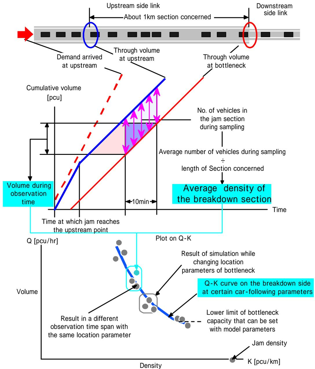
Fig.36 How to determine the Q-K characteristics in the breakdown flow
