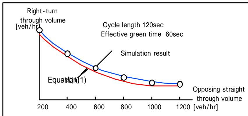
Fig.47 Comparison of simulation result and theoretical values for right-turn capacity
