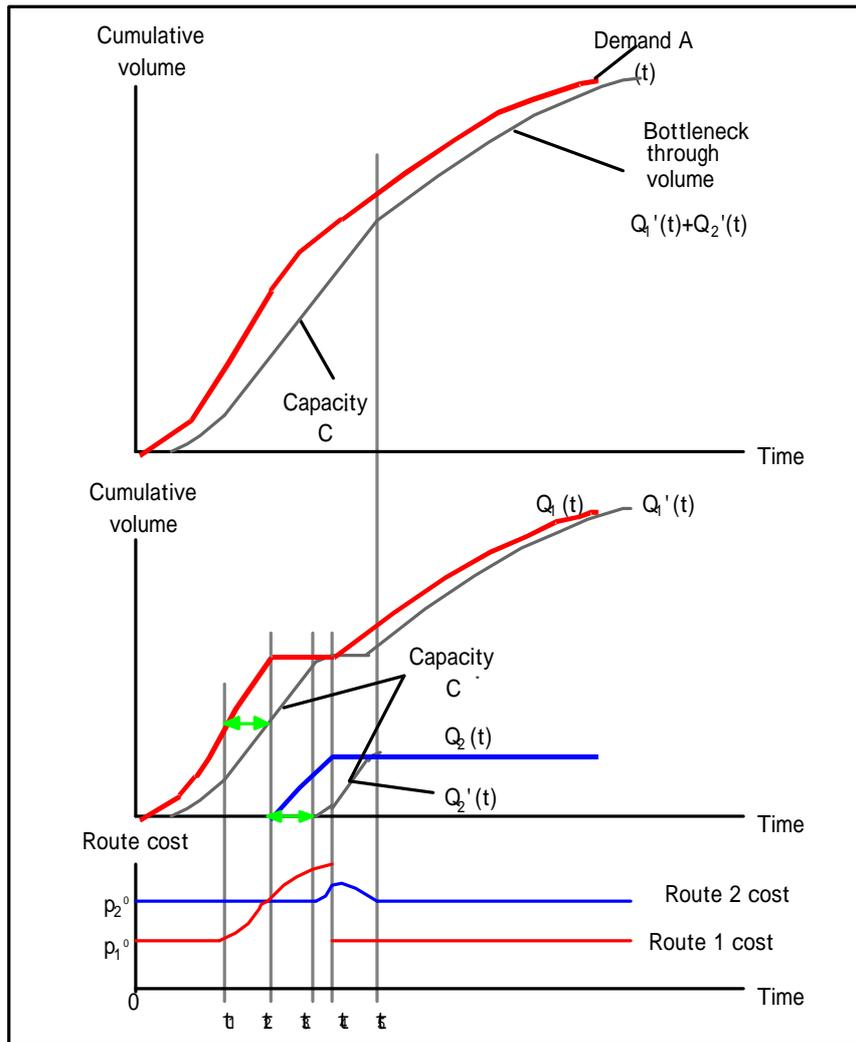
Fig.9 Flow pattern with DUO allocation based on current route required time
