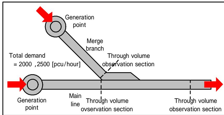
Fig.45 Verification data set for reproducibility of the merge area capacity
