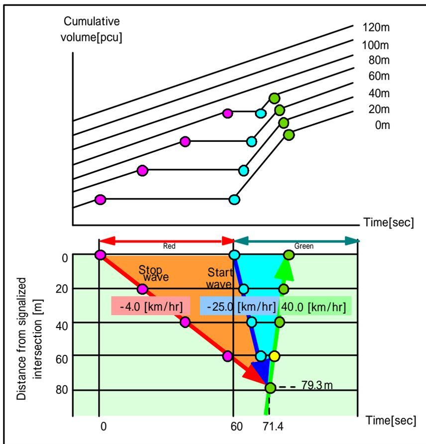
Fig.44 Start/stop wave propagation condition and cumulative volume at each point
