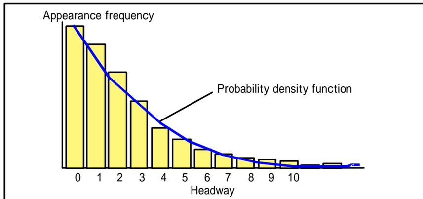
Fig.32 Histogram and theoretical values for headway
