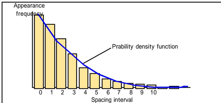
Fig.12 Histogram and theoretical value of headway
