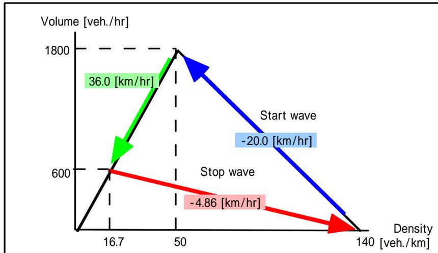
Fig.23 Start and stop wave rate determined from the Q-K curve
