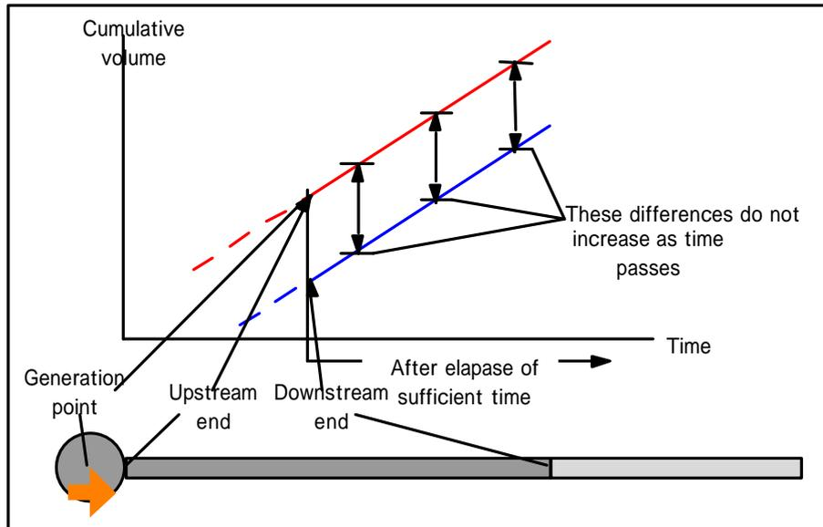
Fig.A1-1 Conceptual view when the free flow is in a steady state
