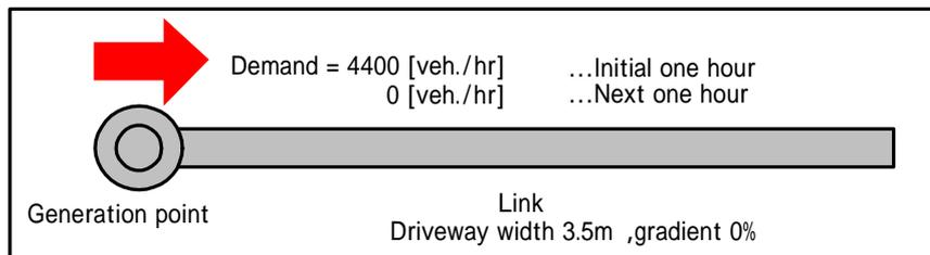
Fig.33 Verification data set for volume conservation when cars in traffic jam are drawn outside the network
