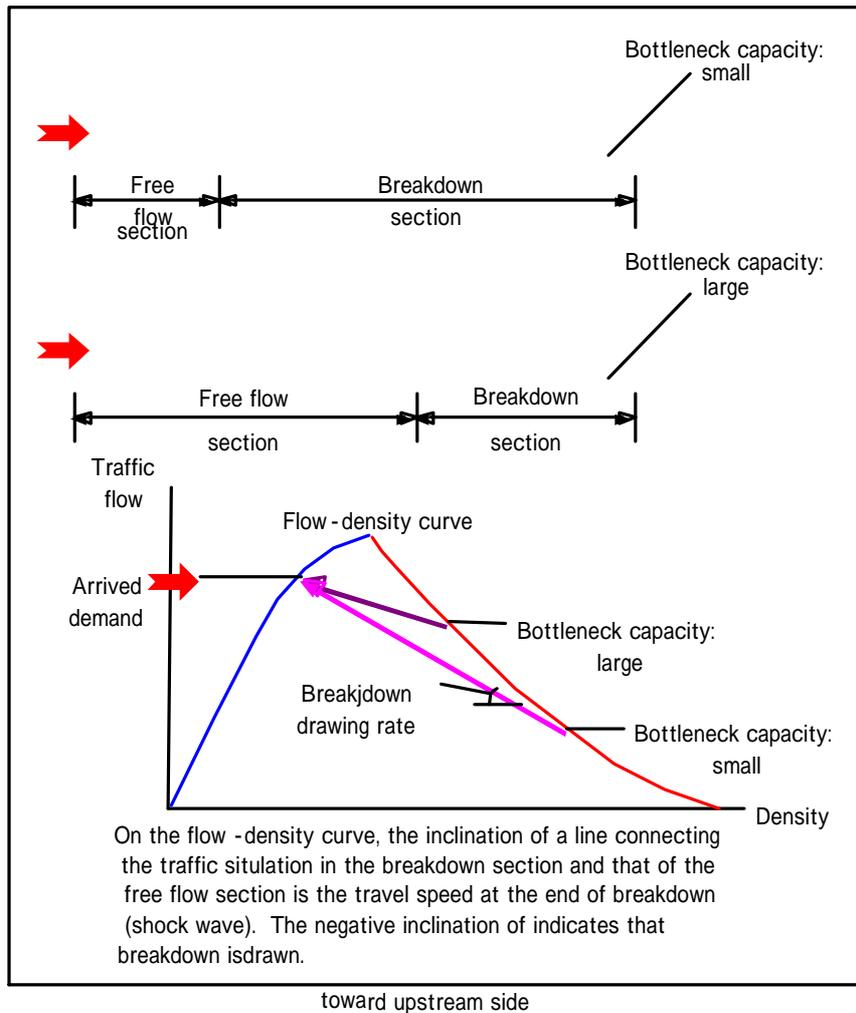
Fig.5 Calculation of breakdown drawing/elimination rate according to the shock wave theory
