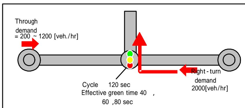
Fig.46 Verification data set for right-turn capacity
