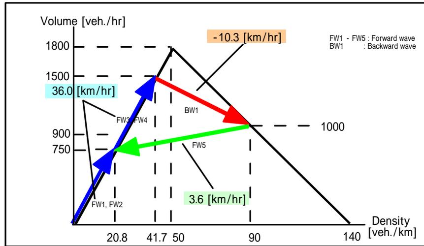
Fig.20 Shock wave propagation rate when the bottleneck capacity is 2000[units/hour]
