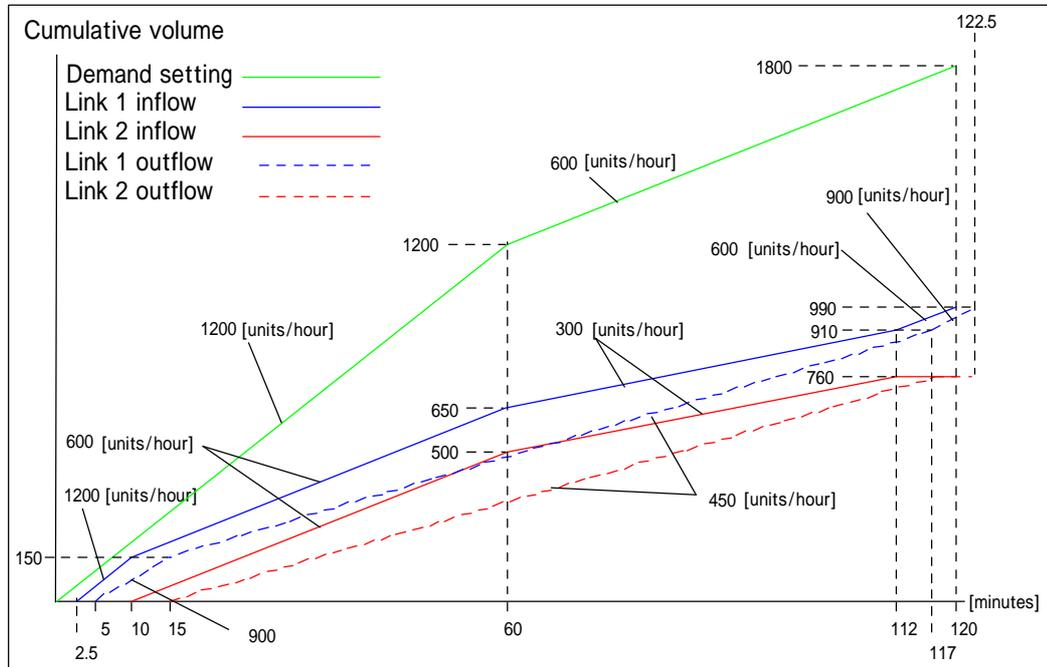
Fig.30 Flow pattern of a case in which DUE is achieved
