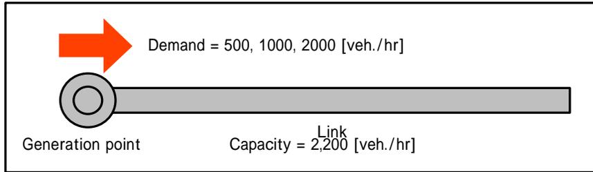
Fig.11 Example of verification data set for vehicle generation model
