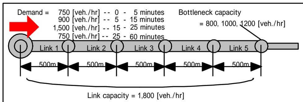
Fig.19 Verification data set for spreading cars out and eliminating traffic jams
