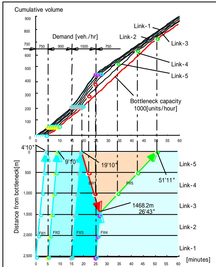
Fig.21 Traffic condition transition diagram on the bottleneck downstream (lower) and observed volume cumulative curve (upper)
