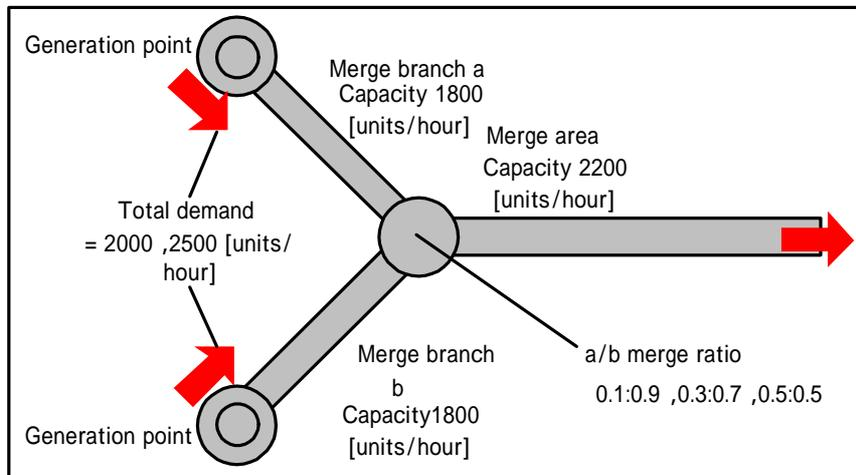
Fig.25 Verification data set for reproducibility of merge capacity
