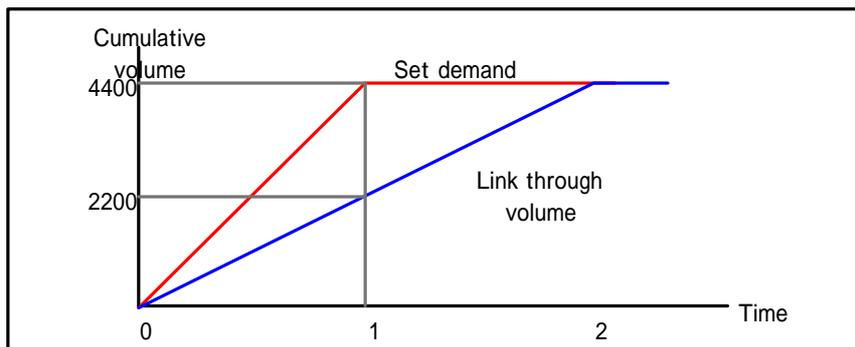
Fig.14 Volume cumulative curve expected when the demand of 4400[units/hour] is given
