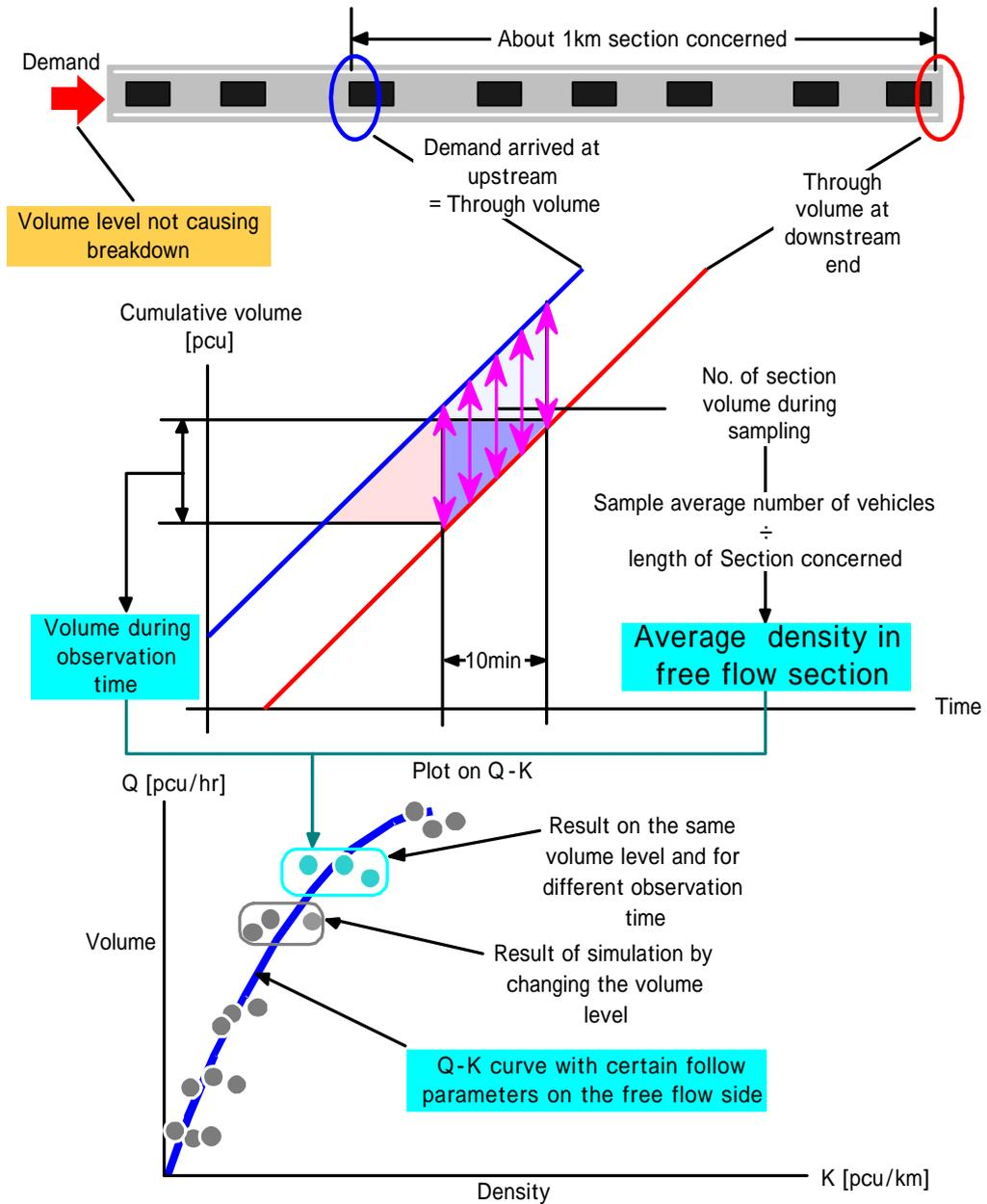
Fig.35 How to determine Q-K characteristics of free flow
