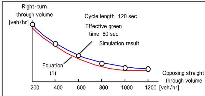
Fig.28 Comparison of right-turn capacity simulation results and theoretical values
