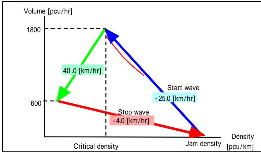
Fig.43 Start/stop wave velocity determined from the Q-K curve
