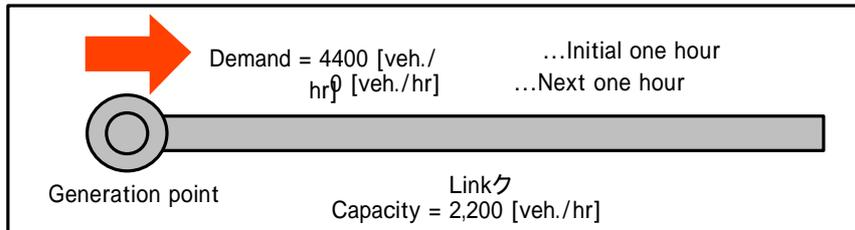
Fig.13 Volume conservation verification data set when cars in a jam are spread out outside the network
